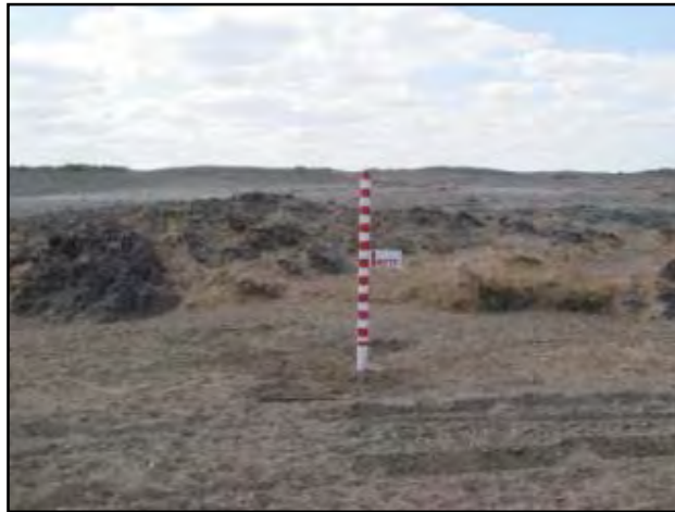
Figure 5.7: Installed flood gauge post on Budaa River, a tributary of the Undai River
