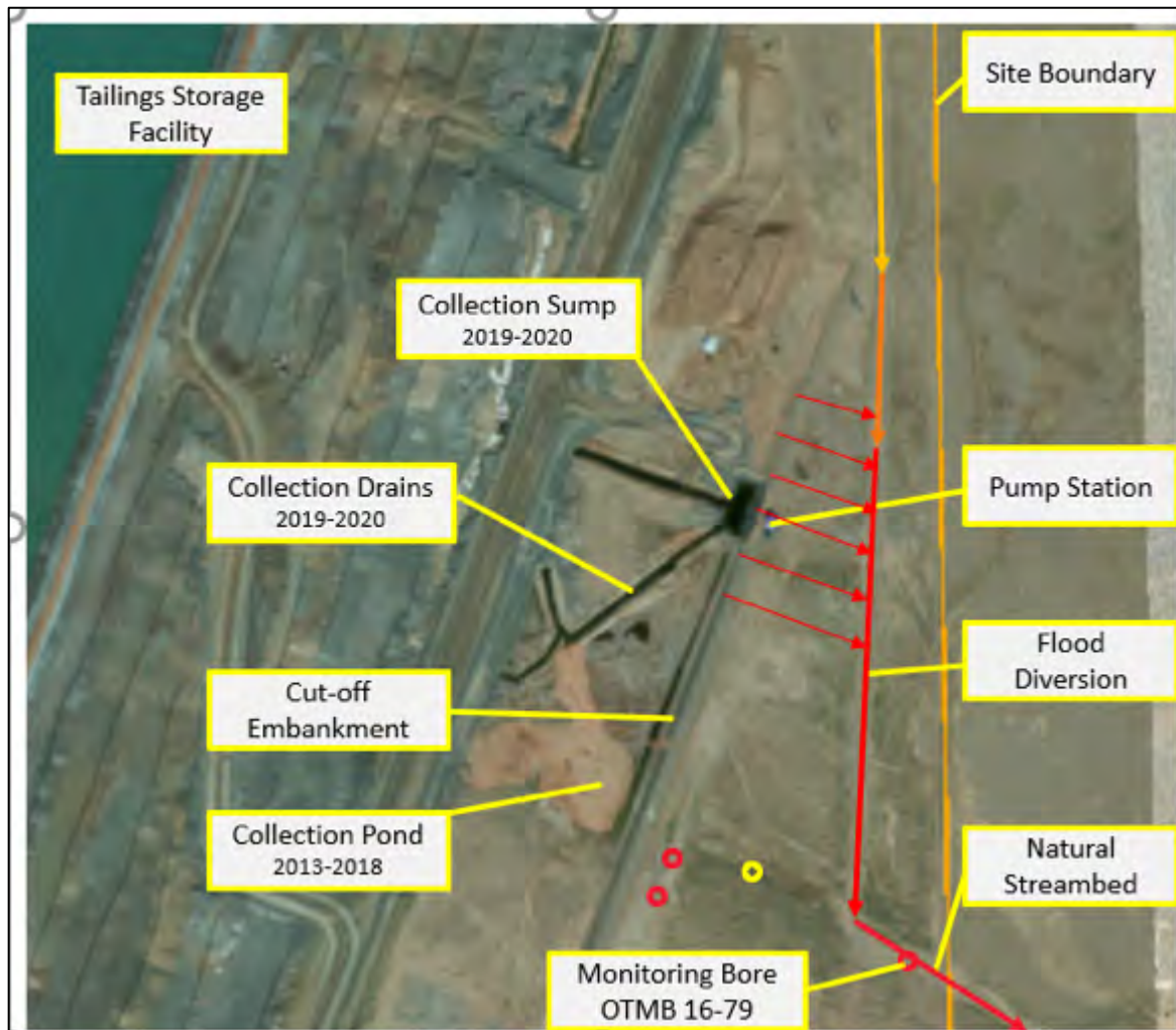
Figure 4-12 Cut-off Dam to the East of the TSF, Location of Historic TSF Seepage Pond/Sump
